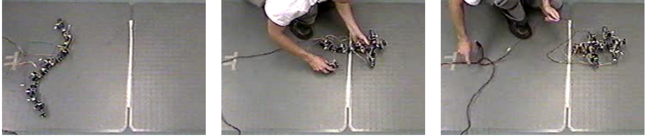
Figure 5: The robot first covers a distance of 63cm using a sidewinder gait (left). The robot is then manually reconfigured into a quadruped walker (middle). Finally the robot walks 87cm (right). Note that the cables only provide power.
