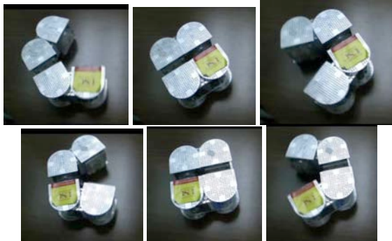
Figure 9: Self-reconfiguration (9a-9f) with SuperBot modules.
