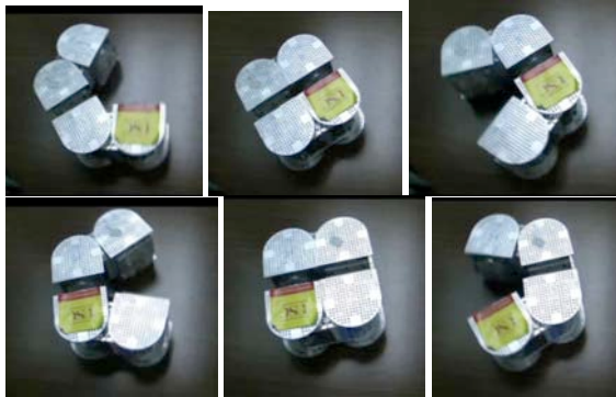
Figure 10: Self-reconfiguration (9a-9f) with SuperBot modules.
