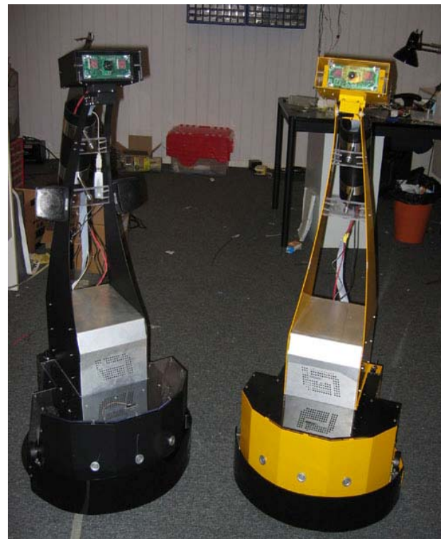
Fig. 1 MILO Personal Robot Platform
