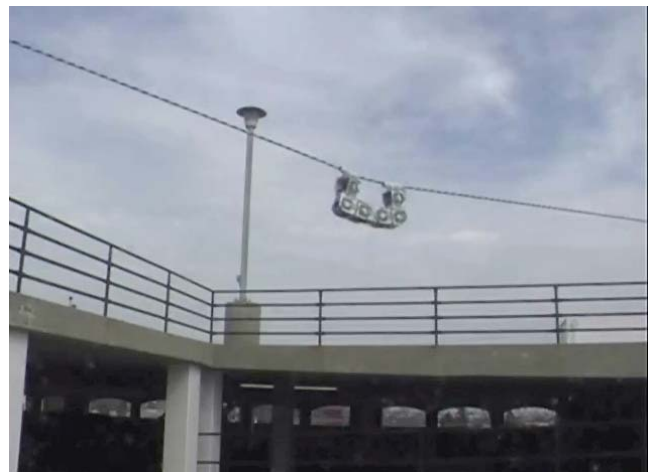
(v) Climbing a 20 meter rope tied around pillars at the top of a structure
