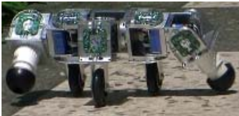
Fig. 3 Front view and back view of tricycleBot gait
