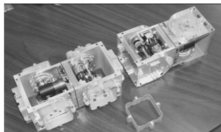
Fig. 1 SuperBot module and connectors
