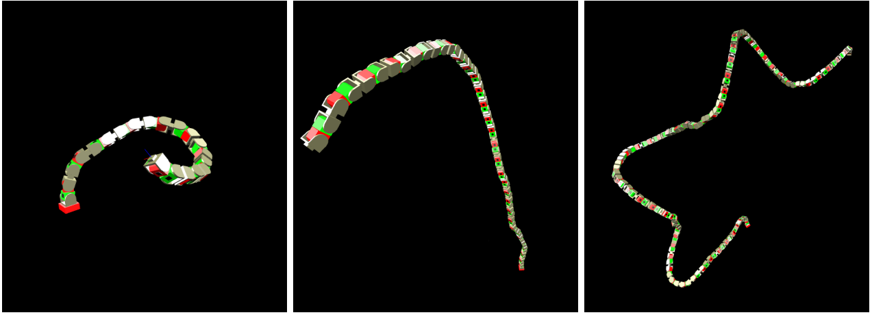
Fig. 1. SuperBot [23] manipulators ranging from 30 to 180 DOF (10-60 SuperBot modules) were used to test PSOIK. Illustrated here are a 30 DOF manipulator (left), a 90 DOF manipulator (middle), and a 180 DOF manipulator (right).
