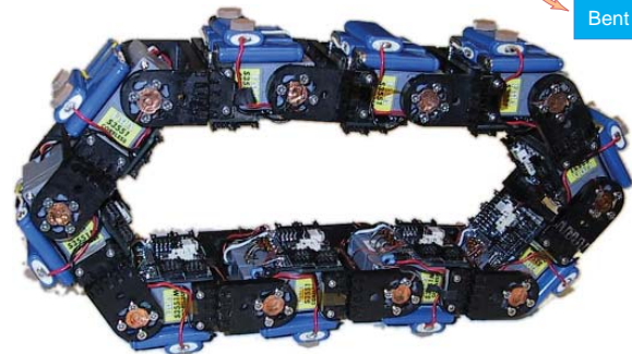
Treading lightly. In "wheel" configuration, Yim's PolyBots move by consulting a gait-control table that cycles each module through four different states.
